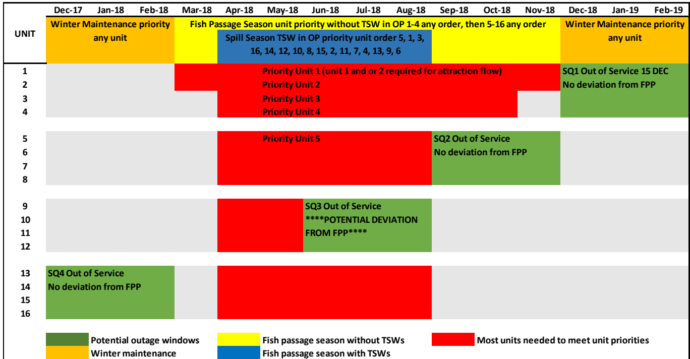
Figure 2. Timeline illustrating unit priorities per the FPP and scheduled SQ board and main unit outages.
